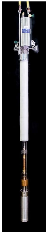
3 He insert 0.3 – 300K or Dilfridge insert 0.05 K – 300K
