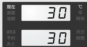
Digital display I: Temperature inside the chamber
