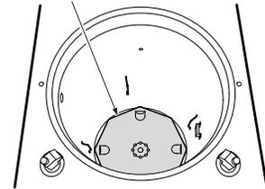
Heater cover Tip (water level) Water level
