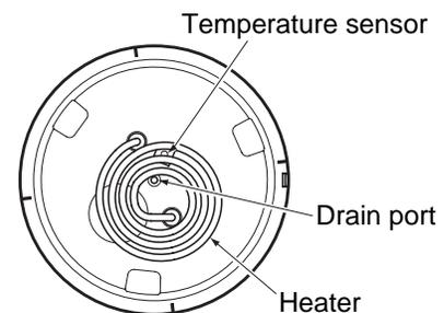
(Plan of bottom of chamber inside)
