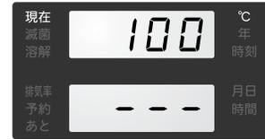
The figure shown above is for the case when the boiling point set temperature is 100°C.
